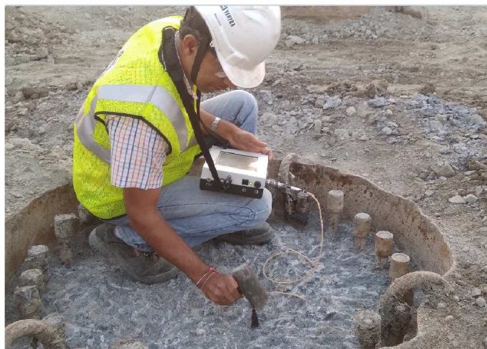
Pile Integrity Test in Progress
